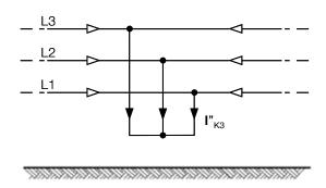
The three-phase short circuit is generally considered as the fault which causes the highest currents (except in particular conditions). In the absence of rotary machines, or when their action is diminished, it also represents the permanent short-circuit current and is the value taken as a reference to determine the breaking capacity of the protection device.
