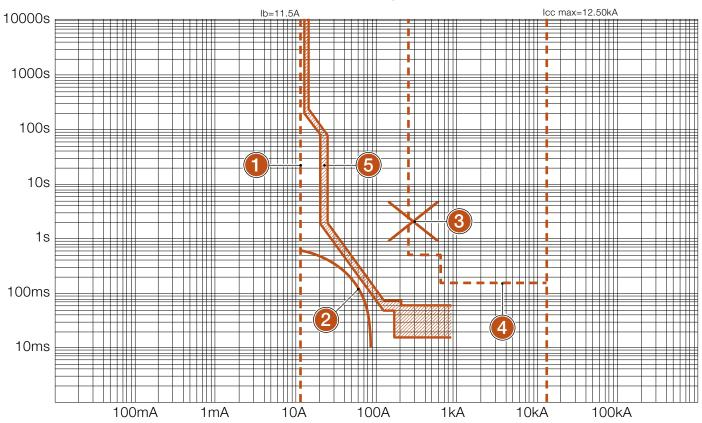
The use of PR221 electronic relays on all the Tmax circuit-beakers of the main LV switchgear in any case guarantees the selectivity of the main LV circuit-breakers with all the outgoing connections to the department switchgear. The following graph shows the curve for the most critical outgoing connection to department A (6).
