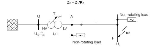
The structure of the electrical network in question can be represented through elements in series; in this way an equivalent circuit is obtained like that shown in the following figure which makes it possible to calculate the equivalent impedance seen from the fault point.
