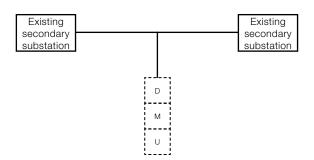
**Scheme E:** Inserting a section of line with a rigid T shunt on an existing MV line only with the circuit-breaker at the network connection system. This scheme is the simplest and least expensive, but reduces the reliability of the networks; it also provides inferior continuity of service. This connection is to be understood as exceptional.
