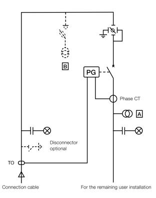
The dashed VT branched on the busbar, indicated by B, is an alternative to the recommended solution indicated by A. As you can tell from the previous figure, the ideal positioning of the homopolar toroid TO is upstream of the DG; the ideal solution both for the inductive CTs and VTs and for the non-inductive transducers is to position them immediately downstream of the DG.
