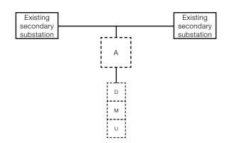
**Scheme C:** Insertion in antenna mode with actuating means (optionally in an additional substation A) along an existing line. From the actuating means, there must be a line dedicated to powering a user. The room possibly dedicated to the actuating means must be able to accommodate the equipment for possible future adoption of in-out insertion.
