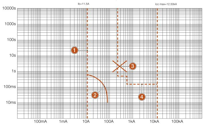
Curve 4 refers to the maximum adjustable values on the protection in accordance with Standard CEI 0-16.
