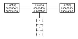
**Scheme B2:** Insertion in antenna mode from a HV/MV substation for connection via a line section connected to the MV busbars of an existing distribution substation. The room dedicated to the network system at the user site must be able to accommodate the equipment for possible future adoption of in-out insertion.
