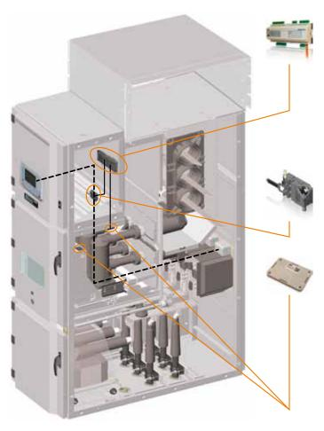
No change is required to the switchgear, the circuit-breaker or the protection relay. The components to be installed are the central unit, the current sensor and the wireless identification device (RDIF) that stores the data of the circuit-breaker in a unique manner and transmits them to the central unit. The predictive algorithms are configured by ABB technicians during installation.
