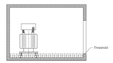
The figure shows a section of the transformer room where the hatched area indicates the containment volume. When disposing of the products of combustion in the event of a fire the Fire Prevention Regulations must be taken into account.
