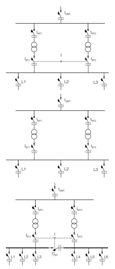
the contribution of other machines. Again in this case, with a transformer out of service, with the possible closure of the coupler, it changes over to a system with a single busbar powered only by the healthy transformer, and load management logic must be provided with disconnection of non-priority loads.
