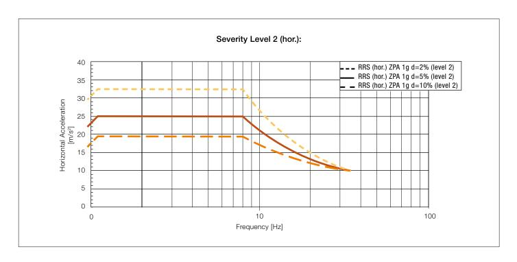
Severity Level 2 (horizonthal) – Zero period acceleration (ZPA) = 1 g
