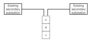
**Scheme A:** Insertion in-and-out mode for connection in the vicinity of an existing line, so as to generate only two line sections belonging to two distinct secondary substations. Under this scheme, the User can be powered again providing better continuity of service.
