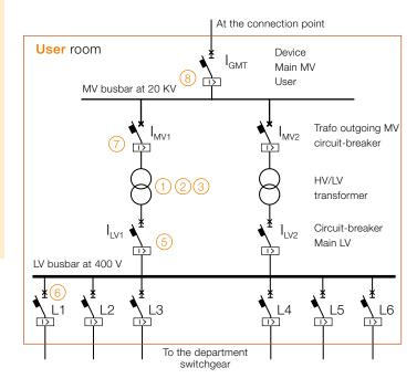
The installation on the MV side consists of an incoming line with a circuit-breaker unit and two transformer outputs equipped with circuit-breakers. The protections, since protection 67N is not required, are of the type REF601, version CEI 0-16.
