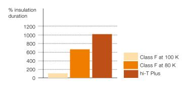
Alternatively, these transformers can be permanently overloaded up to 115% of the rated load, without this having any negative impact on duration. During this overload the maximum temperature of the hot spot would reach 180 °C in accordance with the Standard IEC EN 60076-12.
