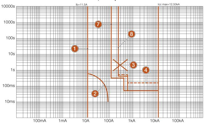
It can be noted that, having already selected an instantaneous value of 0.05 s as the tripping time for the MV transformer protection (7) for the third threshold, it is not possible to obtain selectivity over the whole range of short-circuit currents. Above 600 A, therefore, both the circuit-breakers of the transformers and the DG will trip. However we can
