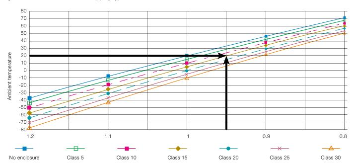
Figure DD.7 - Insulation class 180 °C (H) dry-type transformers load factor in an enclosure
