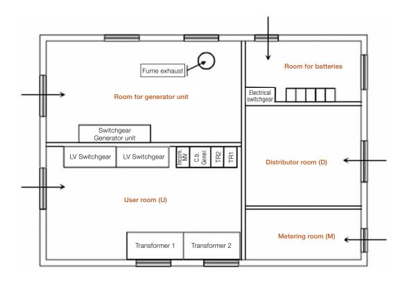
Before positioning equipment inside a substation, you must make sure that the correct distances are observed in the service areas, such as hallways, passages, access and escape routes.
